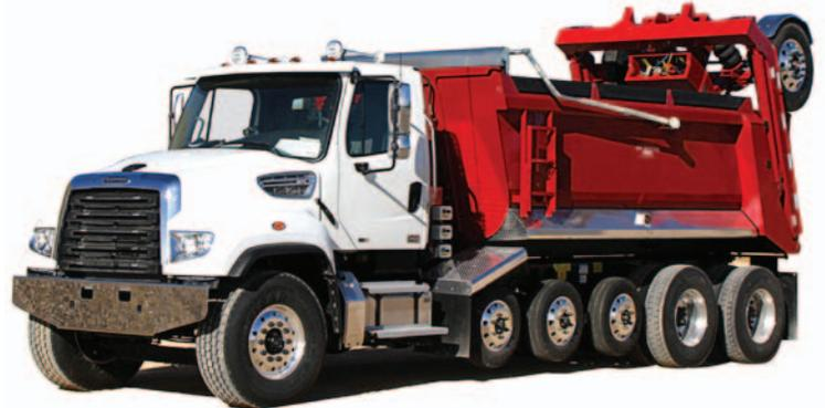
The Ox SuperDump trailing axle configuration allows for bigger payloads with fewer trucks and less trips. For Oldcastle Materials, the SuperDump helps them meet customer expectations with more flexibility.
