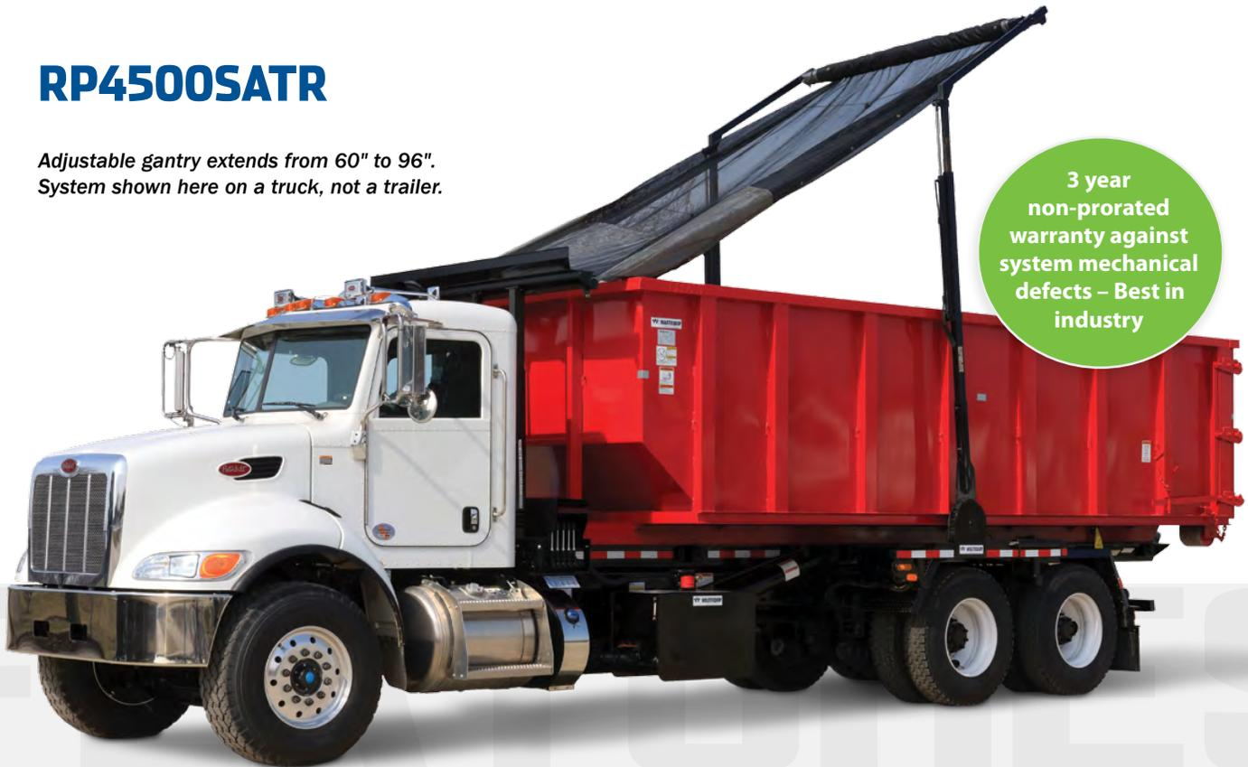
**Rack 'n Pinion STRONG ARM™** systems utilize rack and pinion technology for controlled side arm movement. A hydraulic cylinder moves a rack gear forward and backwards. The rack gear is mated with a pinion gear attached to the base of the pivot arms. This arrangement creates a mechanical advantage which provides continuous control over speed and precise synchronization of the pivot arms as they cover and uncover the container.
