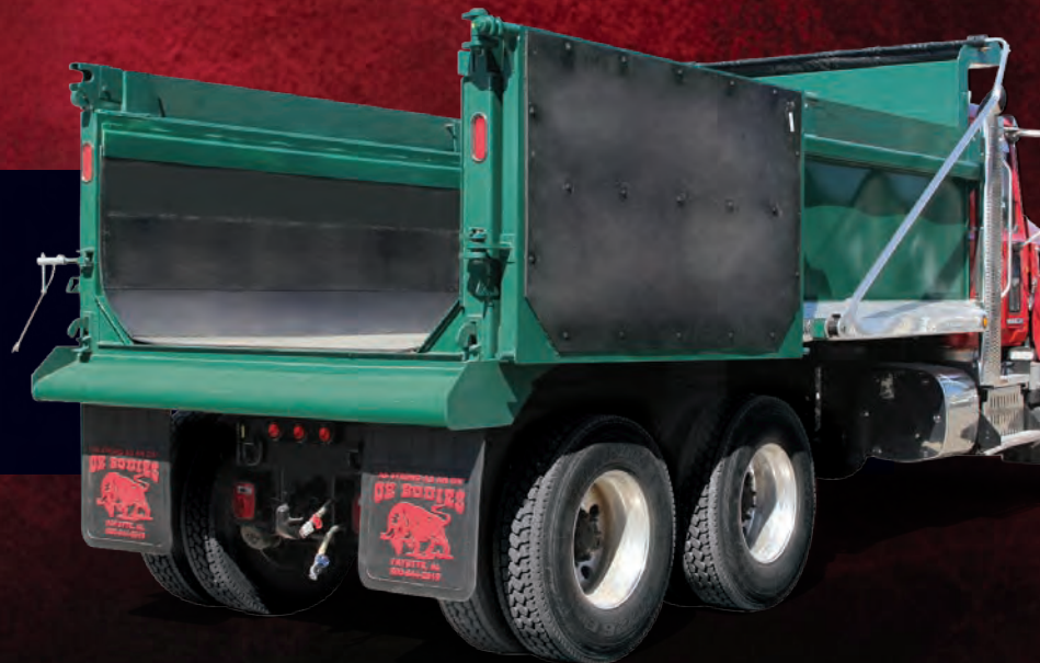
Recessed and rubber grommeted LED lighting to meet FMVSS 108.
