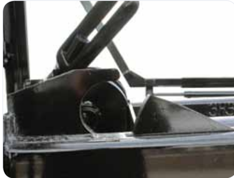
Automatic front container spring-loaded locking system and rear container hold-downs help ensure container remains in place
