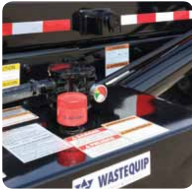
Oil reservoir is filter cart ready, reducing maintenance costs
