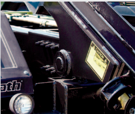
Hoist frame huck bolted to chassis on all factory mounted hoists
