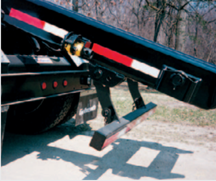
Automatic fold up ICC bumper
