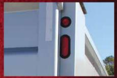
Recessed and rubber grommet mounted LED lighting for side body, tail, clearance, and backup lights to meet Federal standard 108.
