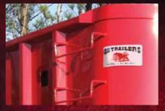
Optional Full body height exterior and internal ladder located on front driver's side.
