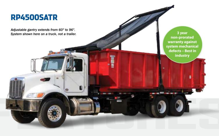
Rack 'n Pinion STRONG ARM™ systems utilize rack and pinion technology for controlled side arm movement. A hydraulic cylinder moves a rack gear forward and backwards. The rack gear is mated with a pinion gear attached to the base of the pivot arms. This arrangement creates a mechanical advantage which provides continuous control over speed and precise synchronization of the pivot arms as they cover and uncover the container.
