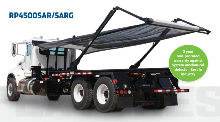
This **Rack 'n Pinion tarp system** has been the system of choice in the roll-off industry for over ten years. Our patented hydraulic arms and gear assembly combined with our Strong Arm technology and Everlast Tarp Roller produce the only fully hydraulic system known for reliability and low maintenance. The Strong Arm concept uses a greatly strengthened base arm which attaches to the Rack 'n Pinion pivot. The extended "C" Channel provides better leverage, greater control and longer life.
