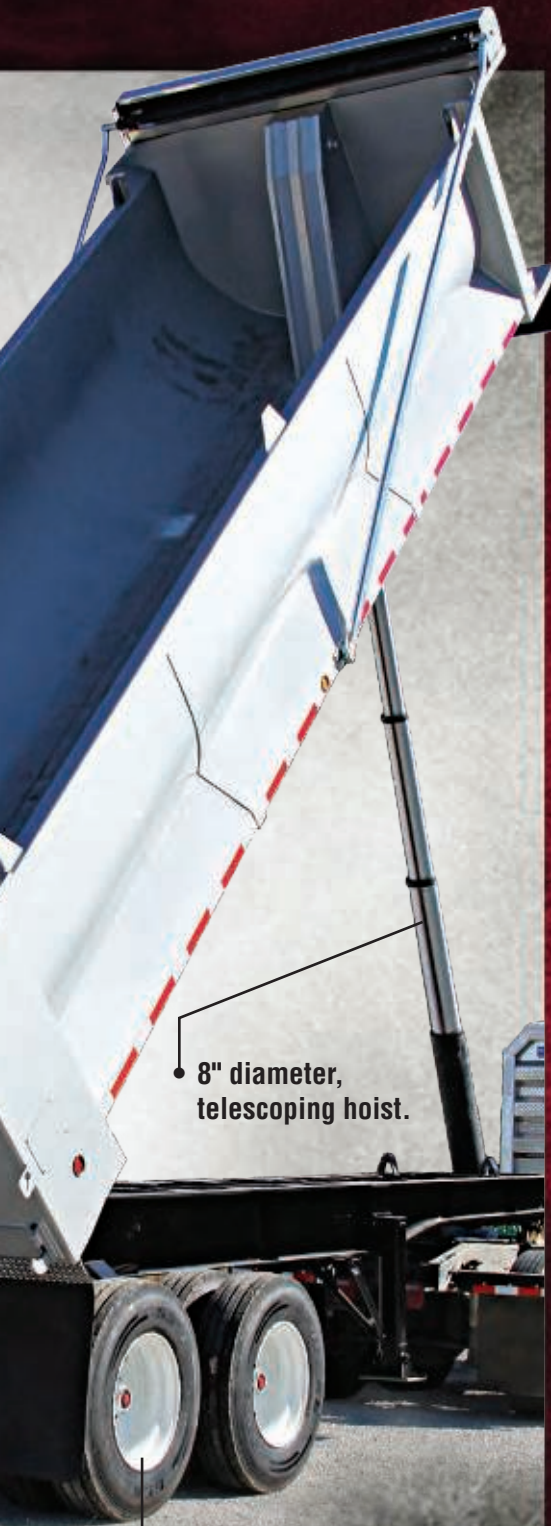
15 x 8.25 wheels with 14-ply tires. Parking system.
