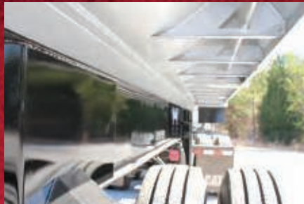
Cross-memberless, 10" I-Beam long sill frame design with Flex Inhibitors. (Elliptical "U" only)
