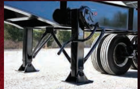
2-speed landing gear.
