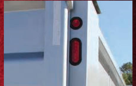
Recessed and rubber grommet mounted LED lighting for side body, tail, clearance, and backup lights to meet Federal standard 108.
