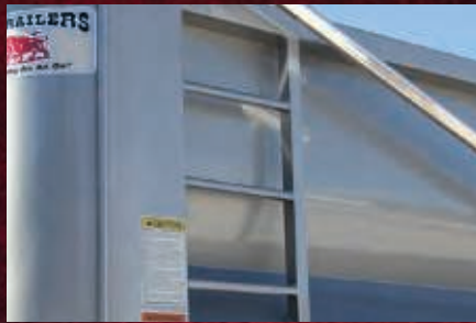
Optional full body height interior and exterior ladder located on front driver's side.
